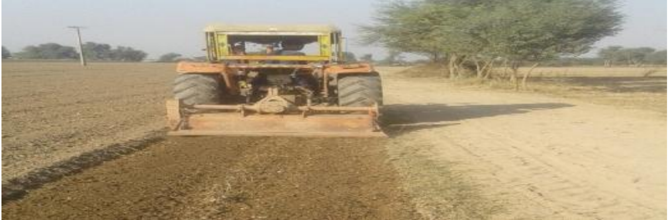
Figure 2. Rotavator in field (Conventional tillage system).
