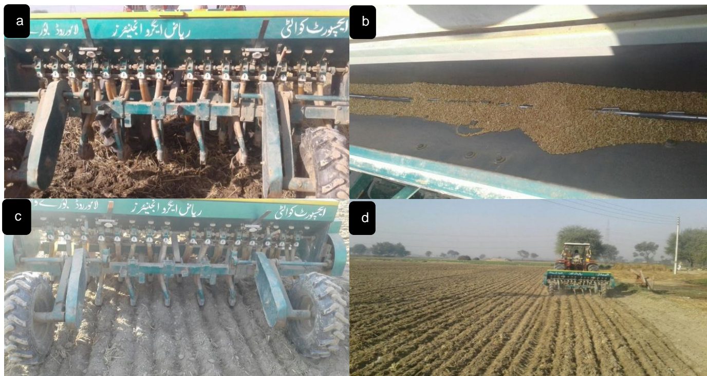
Figure 1. (a) Zero tillage machine in the research area. (b) Physical observation of wheat. (c) Mixing of fertilizer into the soil along with wheat sowing. (d) Wheat sowing using a zero tillage machine.
