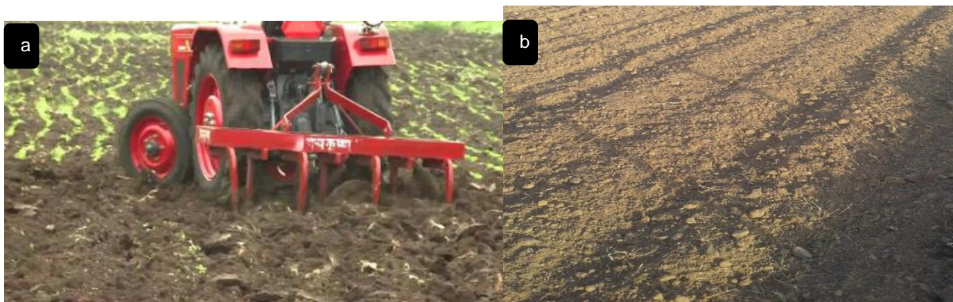
Figure 3. (a) Cultivator in Field. (b) After the utilization of cultivator with planner in field.
